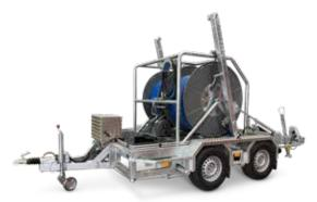
Hydrodiesel delivers a wide range high capacity, ready to use pumps. The pumps are diesel hydraulic driven and therefore do not depend on electricity. The pumps have a displacement capacity of 2 x 2,500 cubic meters per hour (2 x 41,600 liters per minute). That makes a total of 83,200 liters per minute at a head of 17 meters liquid column.
